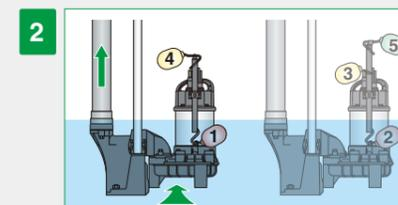
The "A" unit is discharging water (Water level falls).
