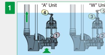
The next time the water level rises, Float #1 on the "A" unit is activated but the unit does not start until Float #4 is activated.
