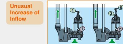
If inflow exceeds the capacity of "A" unit and the water level rises to Float #5, "W" unit starts.
