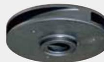
The closed impeller is adopted in the PSF-series. The impeller is also referred to as shrouded impeller, as it has circular shrouds at both sides of the impeller vanes. Although the pump has a limited solids passage capability, it can be used for higher pumping head applications.
