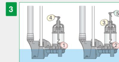
When water level falls and Float #1 is activated, the "A" unit stops. At the same time, "W" unit becomes ready for operation for the next level rise.
