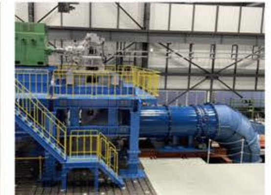
Test-run of a vertical shaft mixed-flow pump with a 1,800 mm diameter
