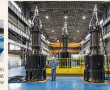
▲ SSP-1350GS submersible column pumps (with a 1,350 mm discharge bore and output of 350 kW), some of the largest pumps of their kind in Japan, helping generate waterflow on an artificial canoe slalom course
