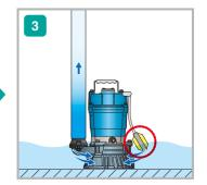
When the water level lowers to the preset level, pump stops operating.
