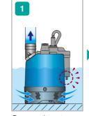
Pump continues to run while the electric probe remains submerged.
