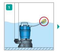
Pump starts operating when the water level rises to a preset level.
