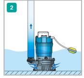
Pump keeps running while the float switch remains on.
